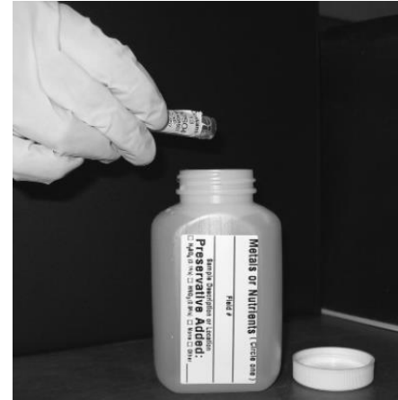
Figure 2. Add a vial of sulfuric acid to sample. Be sure to place cap topside down to avoid contamination.
