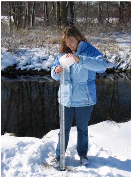
Figure 3. Add small amounts of water to the Transparency Tube until the disk just disappears
