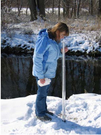
Figure 2. Slowly releasing water with the petcock until the disk is just visible.
