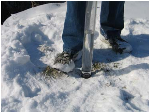
Figure 3. Add small amounts of water to the Transparency Tube until the disk just disappears
