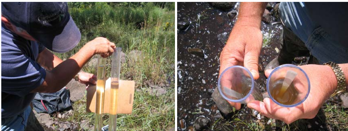
Figure 14: Comparative wall thickness and clarity of transparency tubes. In image a, the Fieldmaster tube is on the right. In image b, the Fieldmaster tube is on the left
