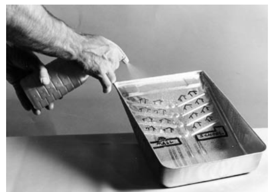
Making rain on the “urban” watershed (number of sprays are again counted).
