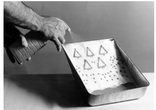
Making rain on the “natural vegetation watershed” (number of sprays are counted).
