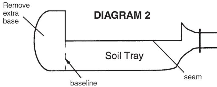
5. Use the marker to draw a line along each seam from the baseline to the neck of the bottle (see Diagram 2).
